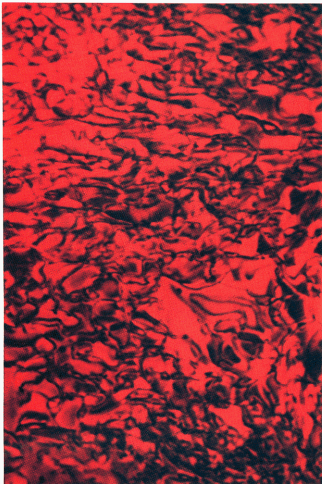
Figure 2. Optical micrograph between cross polarizers revealing a liquid crystalline phase in compound 3 at 164 °C (magnification 320 \times ).
