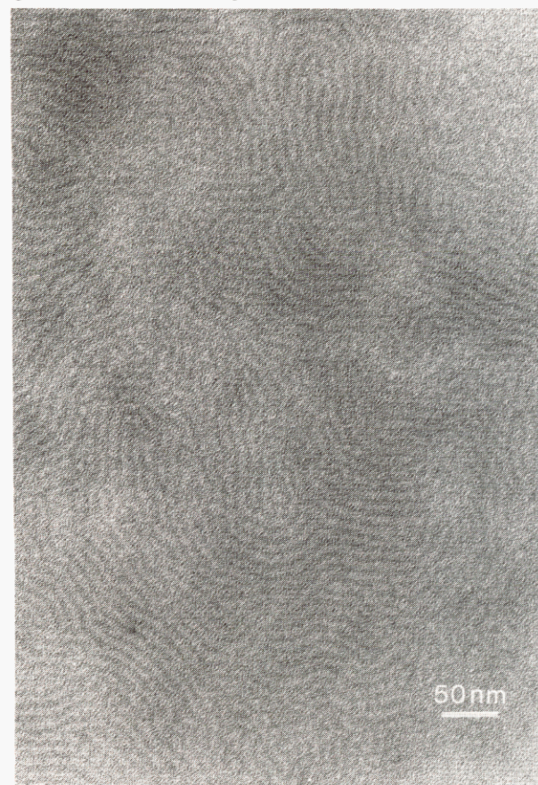
Figure 4. TEM micrograph of rodcoil polymer 5 after annealing at 140 °C for 12 h and staining with OsO 4 . The rod-containing domains have an average thickness of 70 Å.
